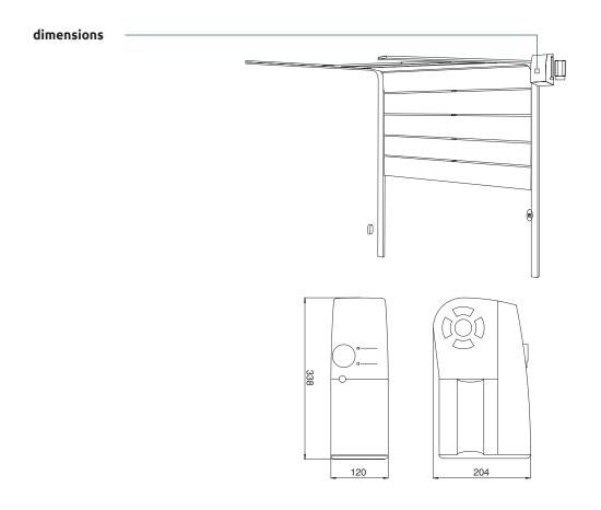
NB. With sectional doors of over 22 sq.m and up to 34 sq.m you need to use the VISCH kit.
